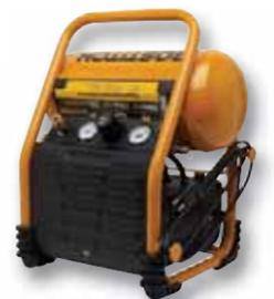
Can be run in either vertical (higher pick-up) or horizontal position (Low CG)
