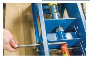
Lubricate the inside of the hose end and/or the shank of the coupling with Dixon's lubricant (DCL-80). Insert the end of the coupling shank into the hose and position the hydraulic ram assembly behind the fitting. Secure the hydraulic ram assembly in place with the position pins. 6.
