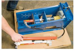
Close the pump valve and pump the ram forward until the coupling is fully inserted. Note: Make sure the fitting is aligned with hose during insertion. Open the pump valve for automatic ram return. Remove assembly.
