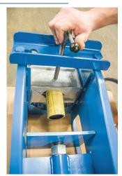
Adjust the hose through the jaw halves such that a sufficient length overhangs to accept the coupling. Turn the threaded spindle to tighten the jaws around the hose.
