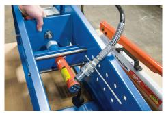
Insert the push plate into the hydraulic ram. Note: The push plate is easily detachable to provide additional room while positioning large hoses and stems.
