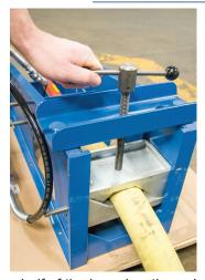
Lower the upper half of the hose jaw through the jaw guides onto the hose.Position the jaw adjustment plate above the top hose jaw.
