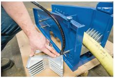
Position the bottom half of the hose jaw \* in the jaw guides such that the hose is in line with the center of the push plate. Secure the bottom half of the hose jaw.
