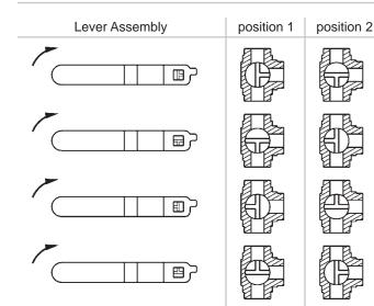
Note: 1/4 turn handle can be adjusted to any orientation. Notches on the valve stem reflect the three openings on the ball.
