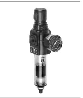
Ordering Information. Models listed include PTF threads, knob adjustment, automatic drain, transparent bowl without guard, 40 µm element, relieving diaphragm, 5 to 150 psig (0.3 to 10 bar) outlet pressure adjustment rang\*, with gauge.
