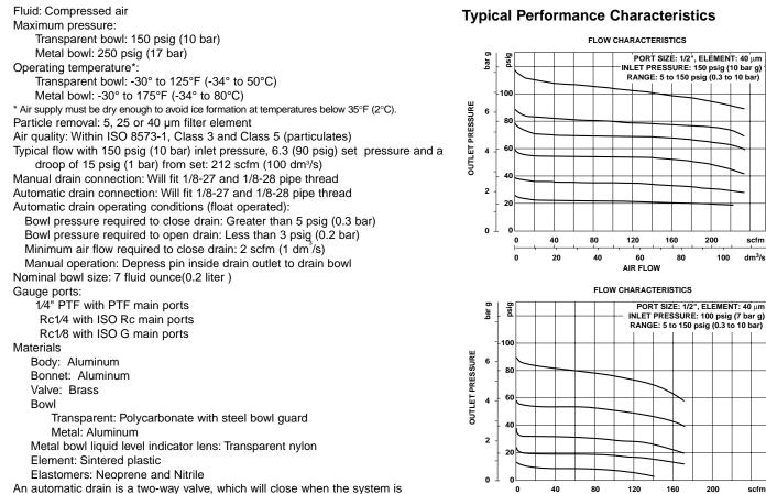
pressurized. The drain opens when the float rises due to accumulated liquid and on depressurization.
