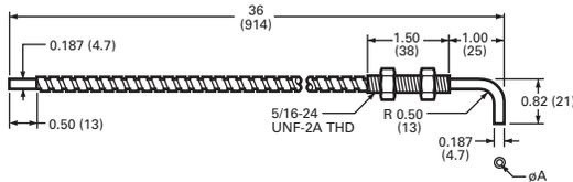
**Right-Angle Viewing, Rectangular Fiber Bundle, Thru-Hole Mounting**
