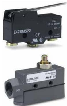
Precision switches are typically available in two types: basic precision and enclosed precision. The basic precision switch is of one-piece construction. The enclosed precision switch is simply a basic switch inside a die cast housing. Basic precision switches are generally not given a NEMA enclosure rating, while some enclosed precision switches can be rated NEMA 4 or 13.
