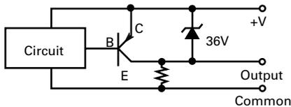
as the output switch. There are two types used, depending on the switching function. One is called **NPN (current sink) open collector**. The output transistor is connected to the negative DC. Current flows from the positive terminal through the load, to the sensor, to the negative terminal. **The sensor "sinks" the current from the load.**
