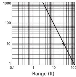
**How to read the gain graph.** If these sensors are spaced 30 ft apart, the excess gain at that distance would be an excess gain of "10".
