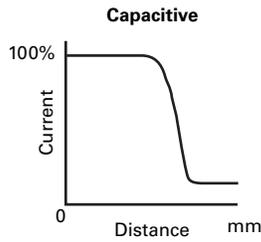
The **output circuit** remains active until the target leaves the sensing field. The oscillator responds with a decrease in amplitude, and when it is no longer receiving sufficient capacitance feedback, the detector circuit switches OFF.
