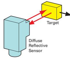
The source and detector elements are mounted in a single sensor housing and are positioned on the same side of the object to be detected and aligned with crossed fields of view. When the target moves into this area light from the source is reflected off the target surface back to the detector and detection occurs. See **Page V8-T12-28**.
