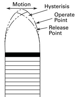
With hysteresis, the **operate point** and the **release point** are **slightly different distances** from the sensor face.
