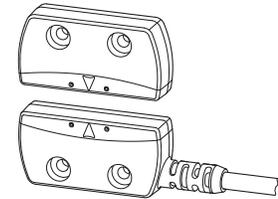
Activation of the non-contact interlock switch occurs only when the corresponding magnetic actuator is within operating range. The actuator is usually mounted on a door or machine guard in such a way that when the door or the guard is closed, the actuator is within operating range and actuates the sensor. The design of the sensor/actuator combination reduces the likelihood of defeating the sensor with a simple magnet.
