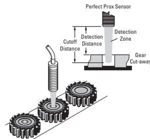
If the hole is present in the gear, the sensor will shine through the hole and ignore the belt—no detection event will occur.
