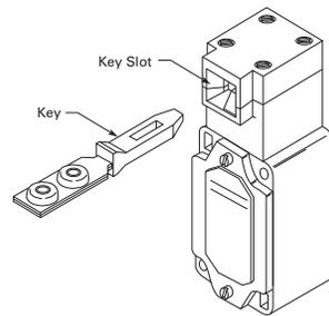
Actuation of the interlock switch occurs only when the corresponding key is inserted into the key slot. The key is usually mounted on a door or machine guard in such a way that when the door or the guard is closed, the key fits into the slot actuating the switch. The special key design makes the safety interlock switch extremely difficult to defeat. When inserted into the slot, the key performs three separate mechanical functions.
