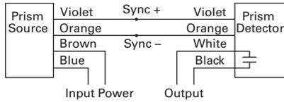
See Prism Series wiring diagrams below for details on wiring power and output.
