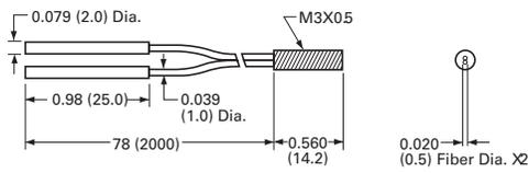
**Small Diameter, Threaded Tip with Bendable Probe**
