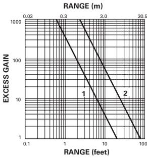
1. 12100A and 12100R detectors using 11100A or 11100R sources
