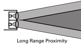
A long-range sensor's source beam and detector's field of view are positioned close together on the same axis. The ability to sense extends quite a distance. **Excess gain peaks out several inches from the sensor, then drops off slowly over distance.**
