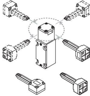
Actuator can be repositioned for horizontal or vertical installation. The operating heads can be rotated manually in 90° steps to suit the specified direction of operation.
