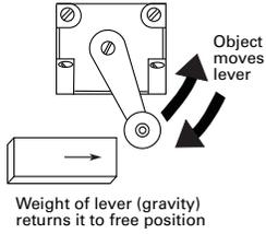
Unlike other rotary limit switches, this switch has no spring return mechanism. **The weight of the operating lever must provide the force to return it to its free position.** This switch is usually mounted with the operating head facing down.
