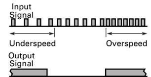
Detects both overspeed and underspeed conditions. The detector is set to count a certain number of objects in a specified amount of time. If the system operates either at a higher or lower rate, an output is generated.
