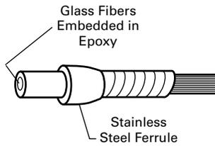
A glass fiber optic cable is made up of a large number of individual glass fibers, sheathed for protection against damage and excess flexing. Plastic fiber optic cables include a single plastic fiber in a protective coating. Neither type of cable contains electronics.
