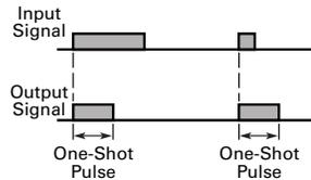
This type of logic generates an output of a set length no matter how long an object is detected. A one-shot can be programmed to trigger on the leading or trailing edge of a target. A one-shot ON signal must time out before it can detect another input.
