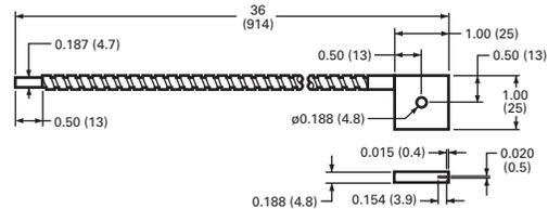
**Right-Angle Viewing, Threaded Cable End**
