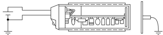
The capacitive proximity sensor has four basic elements: a sensor (which is a dielectric), an oscillator circuit, a detector circuit and an output circuit.
