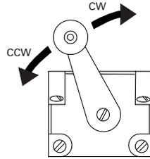
With this limit switch, the **direction of operation can be detected.**
