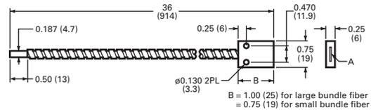
**Right-Angle Viewing, Threaded Cable Shaft**
