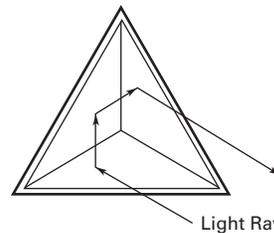
When a ray of light strikes one of the three adjoining sides, the ray is reflected to the second side, then to the third, and then back to its source in a direction parallel to its original course. Thousands of these cube shapes are molded into a rugged plastic reflector or vinyl material.
