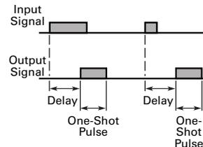
Combines on delay and one-shot logic. The one-shot feature is delayed for a predetermined period of time after an object is detected. A delayed one-shot is useful where the photoelectric control cannot be mounted exactly where the action is taking place. This includes applications like paint booths, high temperature ovens or drying bins.
