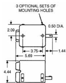
**Pneumatic Time Delay Switches**
