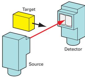
Source and detector elements are mounted in separate housings and aligned facing each other across an area which the target object crosses. Detection occurs when an object blocks the entire effective beam (the column of light that travels in a straight line between lenses). See **Page V8-T12-27**.
