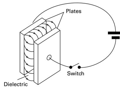
When this principle is applied to the capacitive proximity sensor, **one capacitive plate is part of the switch, the enclosure (the sensor face) is the insulator. The target is the other "plate."** Ground is the common path.
