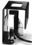
Heavy-duty bracket protects the sensor from damage. Works with all Prism Series sensors. Ideal for material handling applications with Prism right angle reflex sensors. Provides locking vertical and horizontal adjustments for independent adjustment in each axis. Sensor mounts on #4 studs. 10 ga. painted steel | <b>E58KS5200</b>                       |
