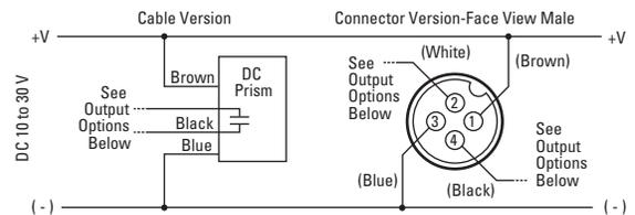
**AC/DC Thru-Beam Wiring**
