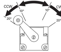
This switch **operates to perform two functions with one switch.** One set of contacts is activated after the lever is rotated 10°, and another set is activated at a 20° rotation (in the same direction).
