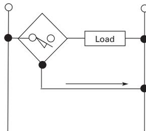
**The operating current the switch pulls from the line, is called the burden current.** This is typically 20 mA. Because the operating current doesn't pass through the load, it is not a major concern for circuit design.
