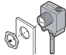
**Mounted SM Sensor in 18 mm Ball Swivel Bracket**
