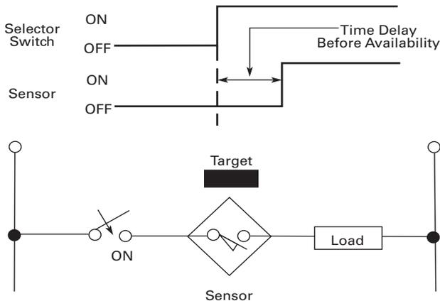
Once the target enters the sensing range and the detector causes the output to change state, a certain amount of time elapses. This
