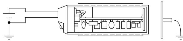
The capacitive proximity sensor has four basic elements: a sensor (which is a dielectric), an oscillator circuit, a detector circuit and an output circuit.
