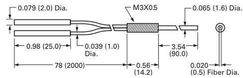
**Pre-Assembled Single Fiber Optic Cables (for Thru-Beam Sensing)**
