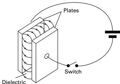
When this principle is applied to the capacitive proximity sensor, **one capacitive plate is part of the switch, the enclosure (the sensor face) is the insulator. The target is the other "plate."** Ground is the common path.
