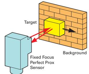
Perfect Prox is a special type of diffuse reflective sensor that combines extremely high sensing power (excess gain) with a sharp optical cutoff. This allows the sensor to reliably detect targets regardless of variations in color, reflectance, contrast or surface shape, while ignoring background objects that are just slightly beyond the target range. See **Page V8-T12-28**.
