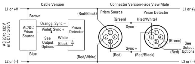
**DC Thru-Beam Wiring**
