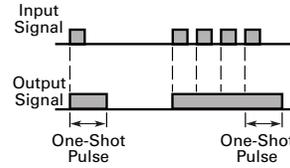
This mode generates an output of predetermined length whenever an object is detected. The sequence restarts each time an object is detected, and will remain triggered as long as a stream of objects are detected before the one-shot times out. A retriggerable one-shot is useful in detecting underspeed conditions on conveyor lines.
