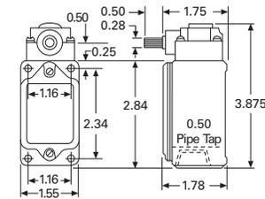
(2) 0.203 Dia. Holes for Front Mtg.
