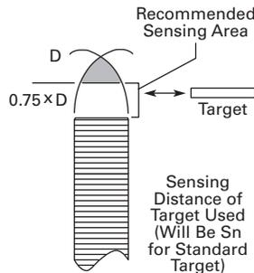
On a slide-by, or **lateral approach**, the target approaches the center axis of the sensing field from the side.
