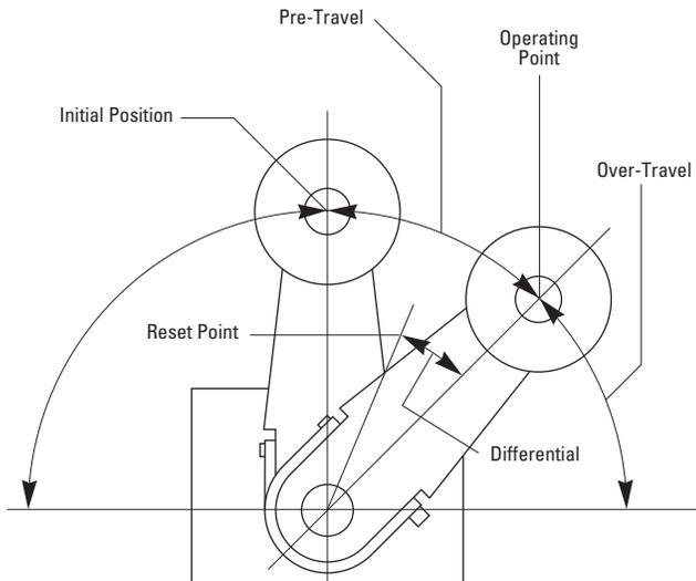
1. The actuator is at its **initial position**. The limit switch contacts are in their normal "untriggered" position.
