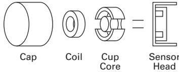
A protective **cap** prevents dust or other environmental hazards from entering the sensor.
