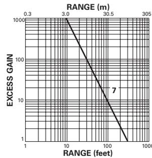
7. E51DEL and E51DED sources using E51DC1 detector
