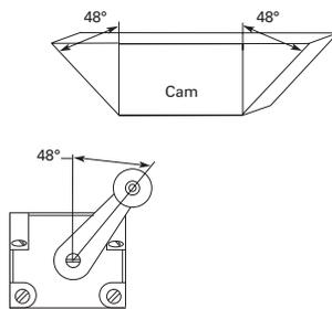
When using side-push or top-push plunger actuators, be sure the cam operates in line with the push rod axis. **Do not use the limit switch body to act as a mechanical stop for the cam in overtravel applications.** Some other type of barrier must be provided as the stop.
