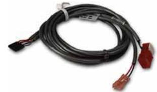
The sensor harness connects the sensor to the buss harness and solenoid<sup>①</sup>. This is the only custom part of the system—the length is optimized for an exact fit on your conveyor to eliminate cable loops that could otherwise be damaged.
