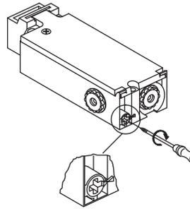
In the event of a loss of voltage, (for example, during commissioning), the spring-powered LS-...-...FT-ZBZ can be released with a screwdriver. **The auxiliary release mechanism must be sealed.**
