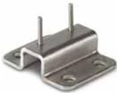
Contoured design is ideal for flush mounting of Right Angle Prism Series reflex to mounting surface using 1/4 in hardware. No alignment adjustment. Sensor mounts on #4 studs. 304 stainless steel                                                                                                                      | <b>6161AS5296</b>                      |
