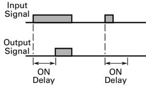
This allows the output signal to turn on only after the target has been detected for a predetermined period of time. The output turns off as soon as the target passes out of range.
