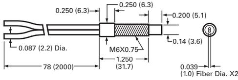
**Large Diameter, Threaded Tip with Bendable Probe**
