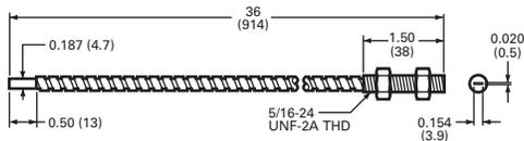
**Forward Viewing, Rectangular Fiber Bundle, Thru-Hole Mounting**
