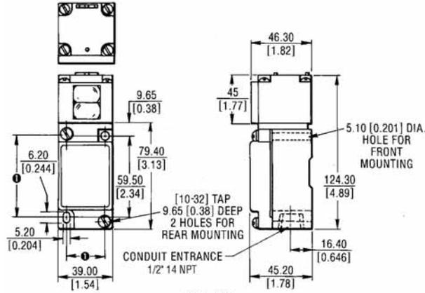
① CAN ACCOMMODATE BOTH U.S. 29.4 x 59.5 [1.16 x 2.34] AND DIN 30 x 60 [1.18 x 2.36] MOUNTING DIMENSIONS.
