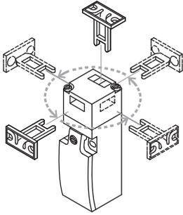
Actuator can be repositioned for horizontal or vertical installation. The operating heads can be rotated manually in 90° steps to suit the specified direction of operation.
