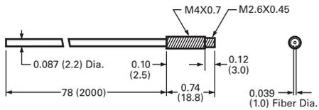
**Large Diameter, Threaded Tip with Bendable Probe**
