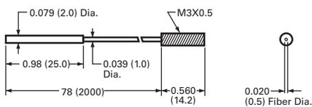
**Small Diameter, Threaded Tip with Bendable Probe**
