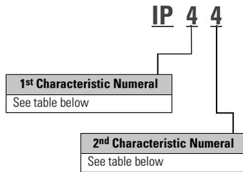
An enclosure with this designation is protected against the penetration of solid objects greater than 1.0 mm and against splashing water.
