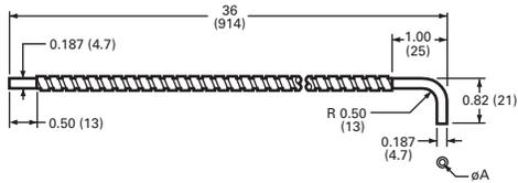
**Forward Viewing, Miniature Probe, Unthreaded**
