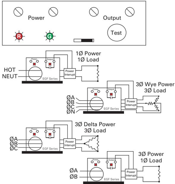
**Mechanical Relay Output Models**
