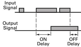
This logic function combines the ON delay logic and OFF delay logic—the output is only generated after the target has been detected for a set period of time, and will remain on after the target is no longer detected for a set period of time.
