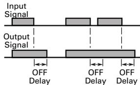
For applications where there is a problem with signal loss in the system, this function turns the output on when the object is detected, and then holds the ON signal for a set period of time after the object is no longer detected.
