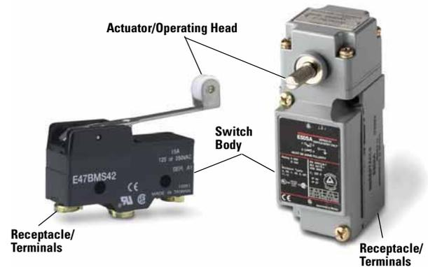
The **actuator** is the part of the limit switch that physically comes in contact with the target. In some limit switches, the actuator is attached to an **operating head**. The operating head translates a rotary, linear or perpendicular "triggering" motion into the motion type needed to open or close the electrical contacts of the switch.
