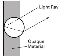
Glass bead retroreflectors are available in tape form for use in dispensers for package coding on conveyors. They are also available in sheet form that can be cut to size. The bead surface is typically rated at 200 to 900 times the reflectivity of white paper.
