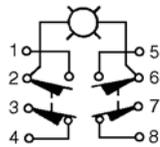
*Parallel wired indicator light. Same polarity each pole.*
