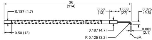
**Forward Viewing, Rectangular Fiber Bundle, Threaded Cable End**
