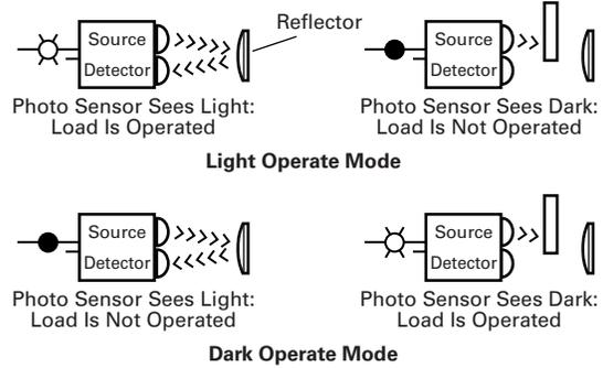
If the control **generates an output when the photodetector does not see light**, the control is said to be working in the **dark operate** mode.
