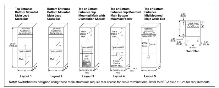
Figure 21.2-5. Main Section Layouts—Dimensions in Inches (mm)
