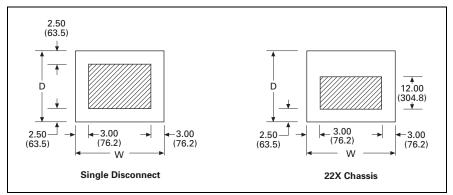
Figure 21.10-23. Typical Conduit Areas—Bottom Cable Exit
