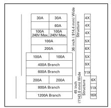
Figure 21.10-22. 22X Chassis Layout Guide-Fusible Switches
