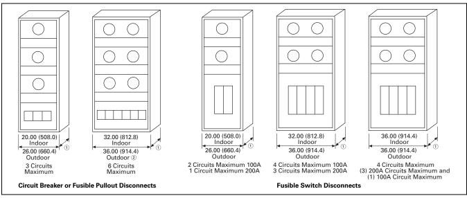
Figure 21.10-5. Tenant Meter and Disconnect Configurations
