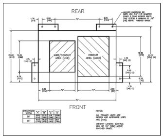
Figure 21.8-1. Bottom View Left Line (Generator) Connection
