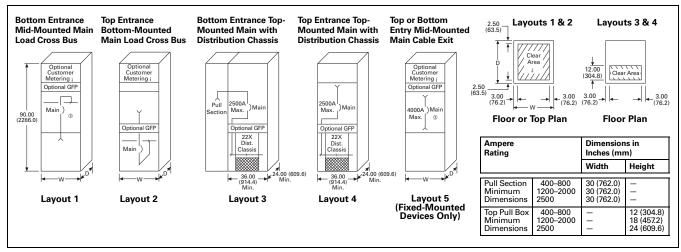
Figure 21.1-5. Main Structure Layouts—Dimensions in Inches (mm)
