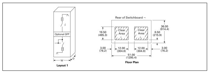
Figure 21.1-12. Individually Mounted Feeder Layout—Dimensions in Inches (mm)
