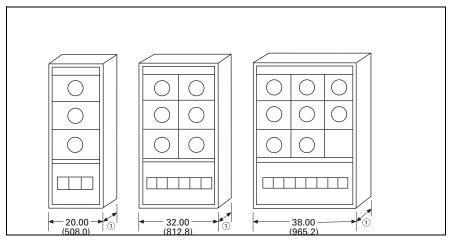
Figure 21.10-14. Circuit Breaker or Fusible Pullout Tenant Disconnects
