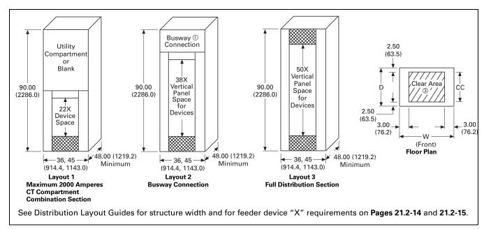
Figure 21.2-10. Distribution Section Layout—Dimensions in Inches (mm)
