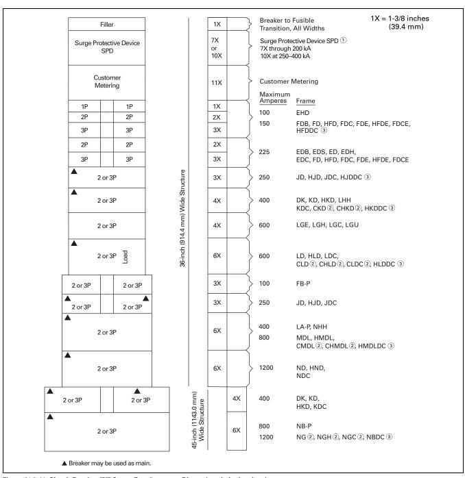
Figure 21.2-11. Circuit Breaker "X" Space Requirement—Dimensions in Inches (mm)
