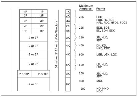
Figure 21.10-24. 22X Chassis Layout Guide—Circuit Breakers, 1X = 1.38 inches (34.9 mm)
