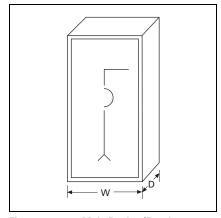
Figure 21.10-12. Main Device (Breaker or Switch)—Bottom Feed
