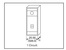
Figure 21.10-19. 400 A Tenant Section with Self-Contained Metering (Breaker)
