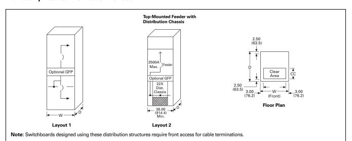
Figure 21.1-6. Individually Mounted Distribution Layouts
