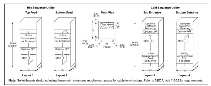
Figure 21.2-4. NEMA Utility Compartment Layouts—Dimensions in Inches (mm)
