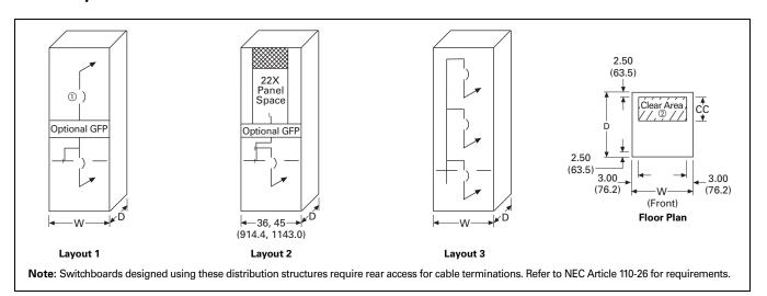
Figure 21.2-7. Individually Mounted Feeder Layouts—Dimensions in Inches (mm)
