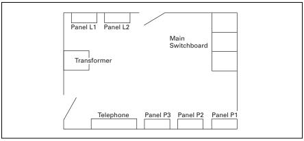
Figure 21.6-1. Traditional Electrical Room—Plan View
