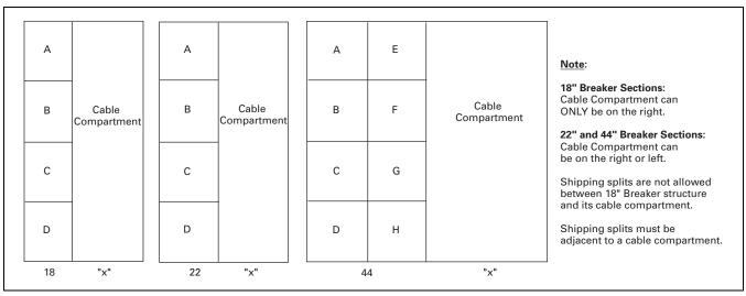
Figure 21.5-3. Breaker Structures
