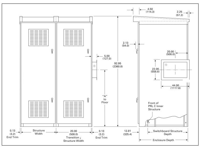
Figure 21.4-2. Front-Access—Non-Walk-In with Sloped Roof—Dimensions in Inches (mm)
