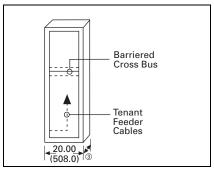
Figure 21.10-17. Load Side Pull Section with Barriered Cross Bus
