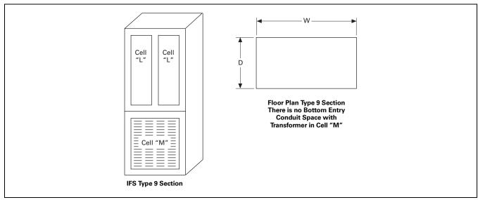
Figure 21.6-8. Type 9 Integrated Facility System Switchboards Distribution Section Layout—Dimensions in Inches (mm)
