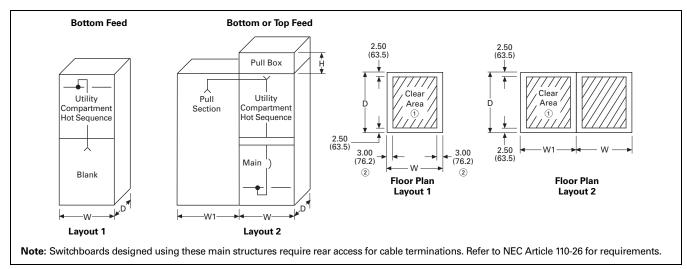
Figure 21.2-3. West Coast Utility Layouts—Dimensions in Inches (mm)
