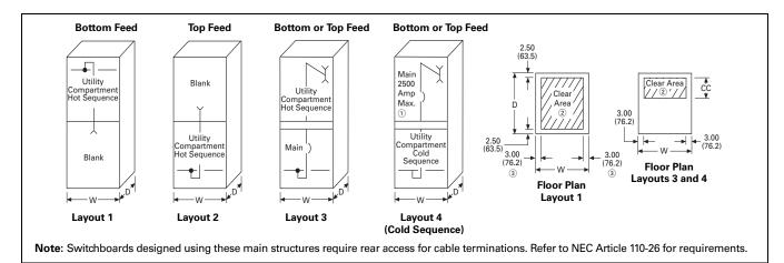
Figure 21.2-2. Utility Compartment Layouts—Dimensions in Inches (mm)
