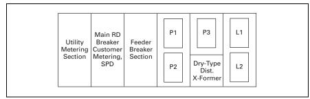
Figure 21.6-3. Optimized IFS Layout—Front View
