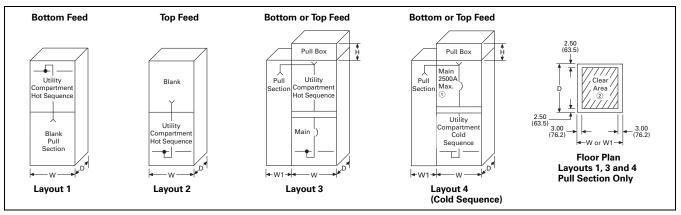
Figure 21.1-2. Incoming Utility Compartment and/or Main Devices—Dimensions in Inches (mm)
