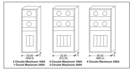
Figure 21.10-15. Fusible Switch Tenant Disconnects
