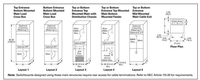
Figure 21.2-6. Main Section Layouts—Dimensions in Inches (mm)
