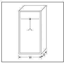
Figure 21.10-2. Main Lugs Only—Top or Bottom Feed
