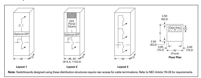
Figure 21.2-8. Individually Mounted Feeder Layouts—Dimensions in Inches (mm)
