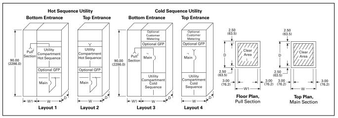
Figure 21.1-4. NEMA Utility Compartment Layouts—Dimensions in Inches (mm)
