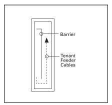
Figure 21.10-8. Rear Barriered Wireway Metering Section Side View
