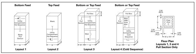
Figure 21.1-1. Incoming Utility Compartment—Dimensions in Inches (mm)
