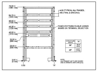
Figure 21.8-2. Front Bus Arrangement
