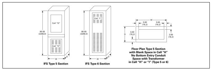
Figure 21.6-6. Type 5 and 6 Integrated Facility System Switchboards Distribution Section Layout—Dimensions in Inches (mm)
