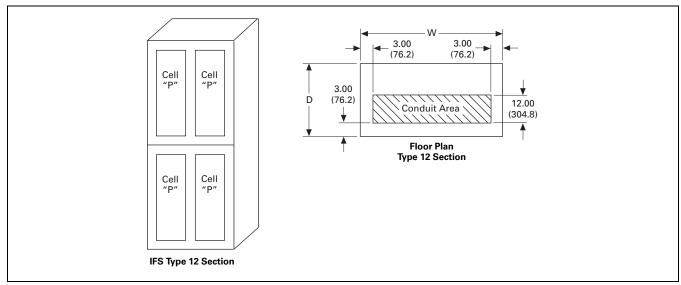
Figure 21.6-10. Type 12 Integrated Facility System Switchboards Distribution Section Layout—Dimensions in Inches (mm)
