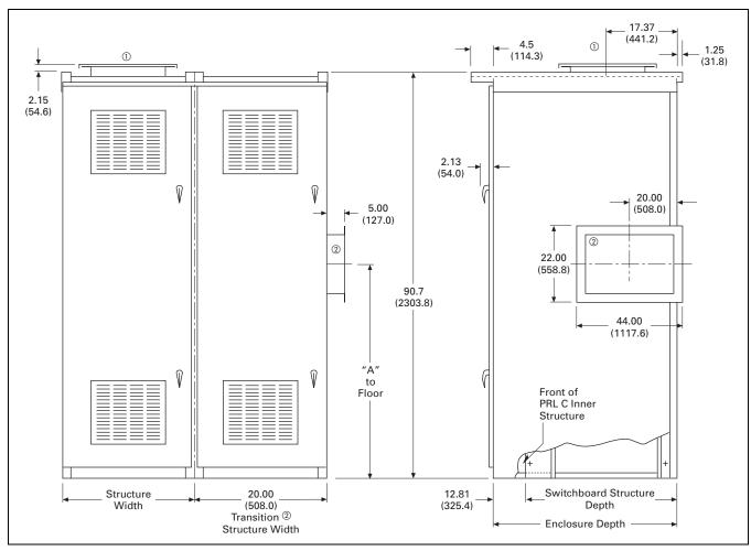
Figure 21.4-1. Front-Access—Non-Walk-In with Flat Roof—Dimensions in Inches (mm)
