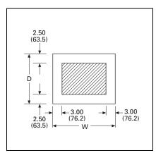
Figure 21.10-1. Typical Conduit Area— Figures 21.10-2, 21.10-3 and 21.10-4
