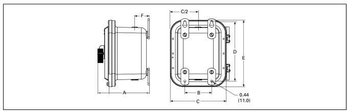
Figure 28.0-25. Non-Fusible and Fusible Disconnect Switch Dimensions
