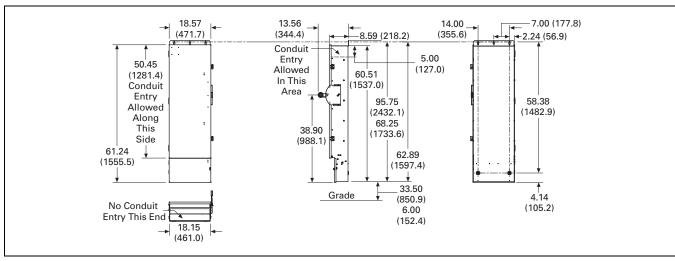
Figure 28.0-15. Quick-Connect Double-Throw 30/200 A—Dimensions in Inches (mm)
