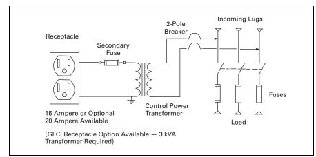
Figure 28.0-3. Auxiliary Power Heavy-Duty Safety Switch Circuit Diagram
