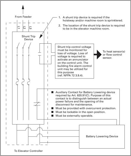
Figure 28.0-2. Shunt Trip Device Wiring Diagram
