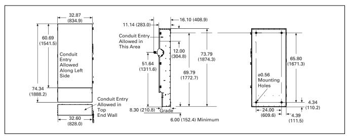
Figure 28.0-20. 400-600 A Quick-Connect Single-Throw Switch—Dimensions in Inches (mm)
