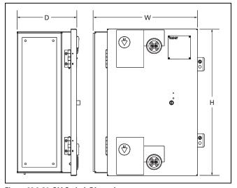
Figure 28.0-24. OLI Switch Dimensions
