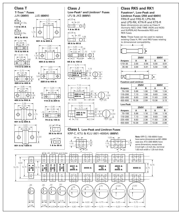
Figure 28.0-26. Typical Fuse Dimensions in Inches
