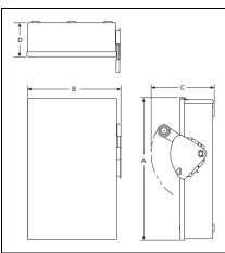
Figure 28.0-13. NEMA Type 3R Dimensions
