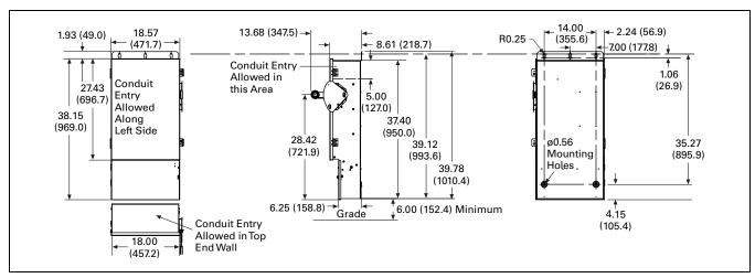
Figure 28.0-18. 100 A Quick-Connect Single-Throw Switch—Dimensions in Inches (mm)
