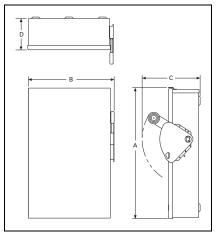
Figure 28.0-11. NEMA Type 3R Dimensions
