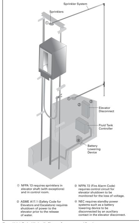
Figure 28.0-1. Typical Hydraulic Elevator Components and Requirements
