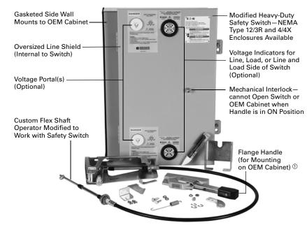
Tlex shaft operator and handle assembly is included and shipped with switch loose, for field installation.
