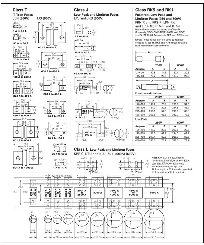
Figure 28.0-27. Typical Fuse Dimensions in Millimeters
