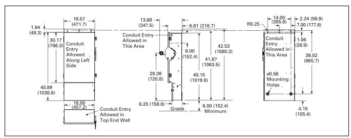
Figure 28.0-19. 200 A Quick-Connect Single-Throw Switch—Dimensions in Inches (mm)
