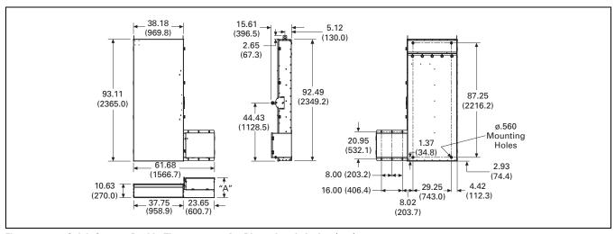
Figure 28.0-17. Quick-Connect Double-Throw 600–800 A—Dimensions in Inches (mm)
