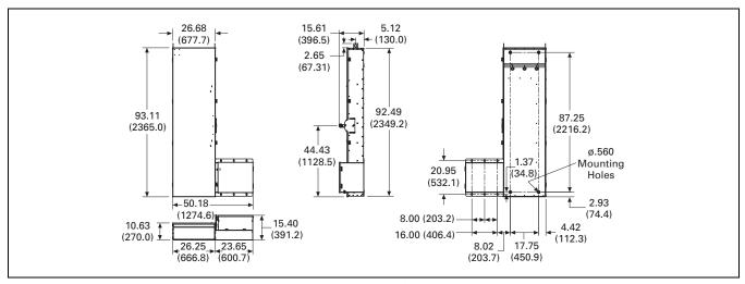
Figure 28.0-16. Quick-Connect Double-Throw 400 A—Dimensions in Inches (mm)
