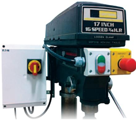
EMS panel shown installed on a drill press.
