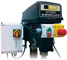
EMS panel shown installed on a drill press.
