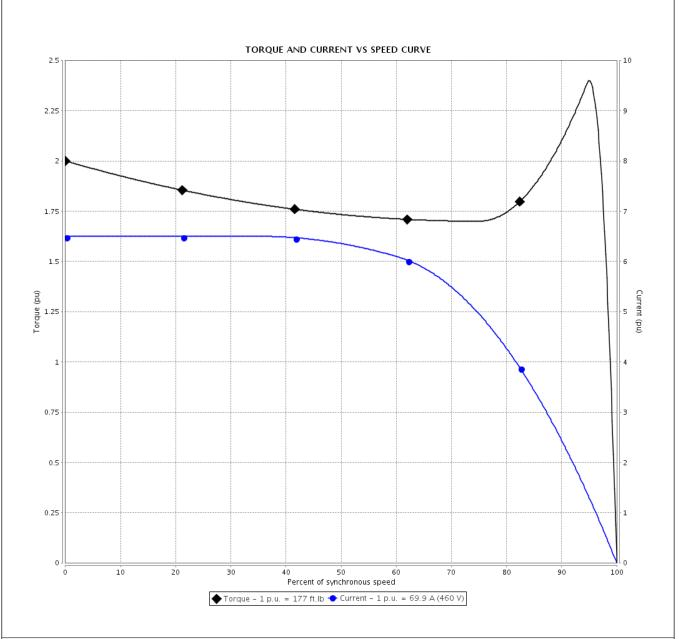
: 460 V 60 Hz 4P Performance Rated current : 69.9 A Moment of inertia (J) : 15.6 sq.ft.lb **LRC** : 6.5 Duty cycle : Cont.(S1) : 177 ft.lb Insulation class Rated torque : F Service factor Locked rotor torque : 200 % : 1.25 Breakdown torque : 240 % Temperature rise : 80 K Rated speed : 1780 rpm Design : B
