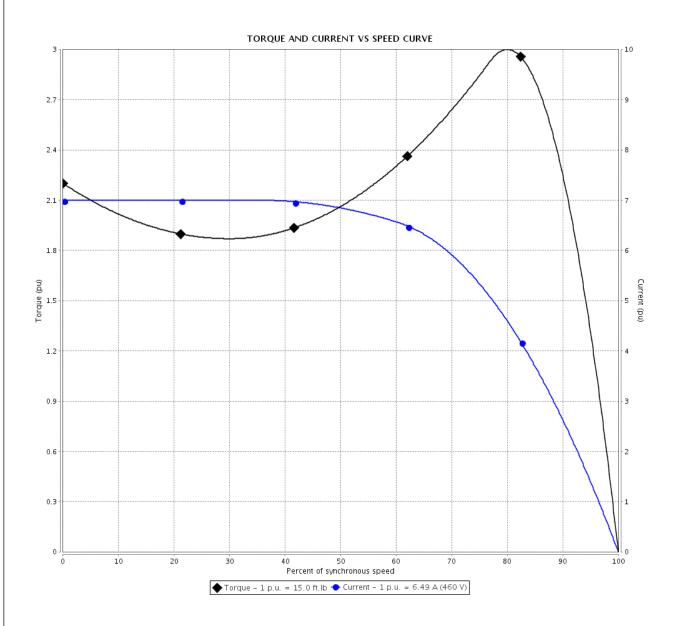
Performance : 230/460 V 60 Hz 4P Rated current : 13.0/6.49 A Moment of inertia (J) : 0.3080 sq.ft.lb **LRC** : 7.0 Duty cycle : Cont.(S1) : 15.0 ft.lb Insulation class : F Rated torque Locked rotor torque : 220 % Service factor : 1.15 Breakdown torque : 300 % Temperature rise : 80 K Rated speed : 1750 rpm Design : B
