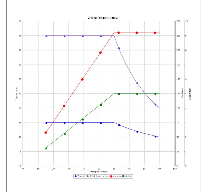
Performance : 230/460 V 60 Hz 4P : 13.0/6.49 A Rated current Moment of inertia (J) : 0.3080 sq.ft.lb **LRC** : 7.0 Duty cycle : Cont.(S1) Insulation class : F Rated torque : 15.0 ft.lb Locked rotor torque : 220 % Service factor : 1.15 Breakdown torque : 300 % Temperature rise : 80 K Rated speed : 1750 rpm Design : B Performed Checked Rev. **Changes Summary** Date Performed by Checked by Revision Page
