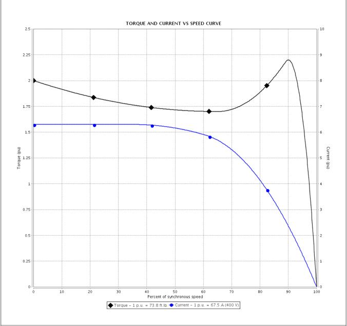
: 200/400 V 60 Hz 2P Performance Rated current : 135/67.5 A Moment of inertia (J) : 3.02 sq.ft.lb **LRC** : 6.3 Duty cycle : Cont.(S1) : 73.8 ft.lb Insulation class Rated torque : F Service factor Locked rotor torque : 200 % : 1.25 Breakdown torque : 220 % Temperature rise : 80 K Rated speed : 3560 rpm Design : B
