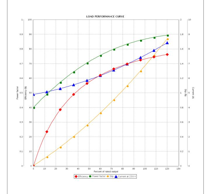
Performance : 230 V 60 Hz 2P : 7.51 A Rated current Moment of inertia (J) **LRC** : 12.2 : Cont.(S1) Duty cycle : 2.22 ft.lb : F Rated torque Insulation class : 1.00 Locked rotor torque : 509 % Service factor Breakdown torque : 250 % Temperature rise : 105 K Rated speed : 3550 rpm
