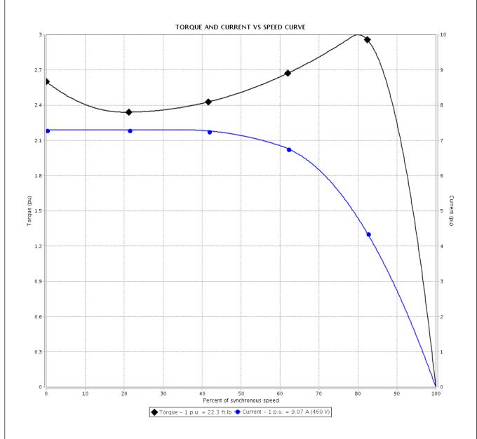
Performance : 230/460 V 60 Hz 4P Rated current : 18.1/9.07 A Moment of inertia (J) : 0.9380 sq.ft.lb **LRC** : 7.3 Duty cycle : Cont.(S1) Insulation class : F Rated torque : 22.3 ft.lb : 260 % Locked rotor torque Service factor : 1.15 Breakdown torque : 300 % Temperature rise : 80 K Rated speed : 1770 rpm Design : B
