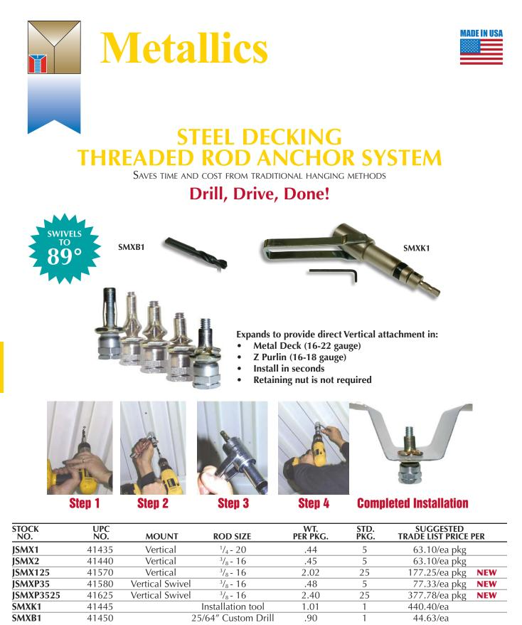
Bit for Tool Installation Kit Includes: Sleeve, bit receiver, hex wrench, and 25/64" drill bit
