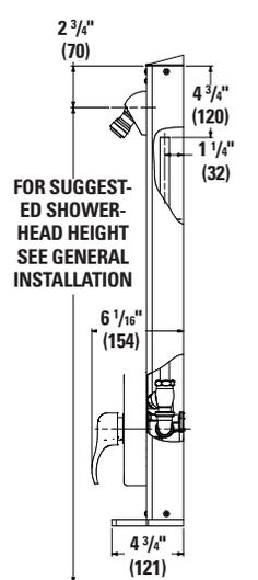
Figure 2: Side dimensions, HydroPanel II Model 450-4210E
