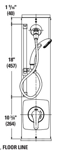
Figure 3: Front dimensions, HydroPanel II Model 450-4214E
