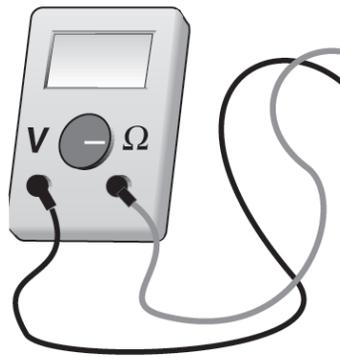
2) using an AC voltmeter. The reading should be between 108 and 132 VAC.
