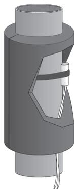
The Supply Sensor should be placed downstream of a circulator pump or after an elbow or similar fitting. This is especially important if large diameter pipes are used, as the thermal stratification within the pipe can result in erroneous sensor readings. Proper sensor location requires that the fluid is thoroughly mixed within the pipe before it reaches the sensor. When using the Supply Sensor with a Mixing Station, insert the sensor into the immersion well, see image below.
