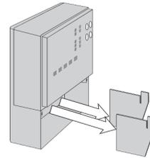
4. Press release clip on base and slide control upward.
