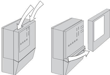
2. Loosen screws at front and pull wiring cover straight out.
