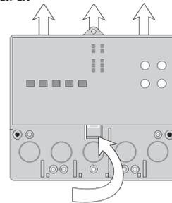
5. The control lifts up and away from the base, which is ready for mounting.
