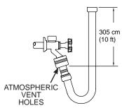
Maintain the hose at a height of 305-cm (10 feet) for five minutes while watching the atmospheric vents for leakage.\*
