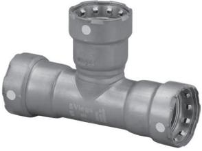
Viega MegaPressG is a carbon steel, cold press system designed for use in compressed air, fuel gas, and heating oil applications. Viegga MegaPressG fittings are designed for use in piping systems utilizing ASTM A53, A106, A135 and A795
