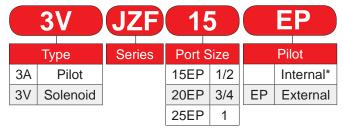
\*Internal Pilot only suitable for pressure operation. Vacuum applications require external pilot models (EP).
