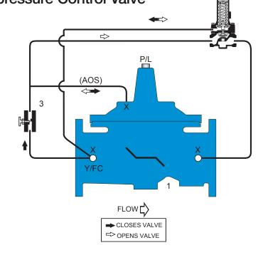
The valve will close, if necessary, until upstream pressure is above the pilot setting. The valve should be specified to include the optional opening speed control and position indicator when used for Pressure Sustaining applications.
