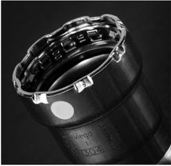
MegaPress 304 FKM fittings are designed to be used with standard IPS ASTM A312 stainless steel pipe to form a complete press system that is ideal for industrial applications. MegaPress 304 FKM ½" to 2" fittings can be used with Schedule 5 to Schedule 40
