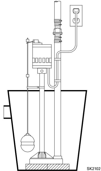
NOTE: This unit is designed for indoor applications where the motor is mounted above the pit cover and protected from water, water spray, and high humidity. Pump is not intended for use with flammable liquids.
