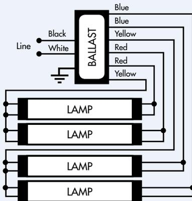
Note: For three lamp operation, cap any blue lead, insulate to 600 volts
