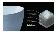
**GALALINE® MATERIAL** Offering outstanding durability, the tub is made of Galaline artificial marble and constructed using TOTO's innovative sandwich configuration.
