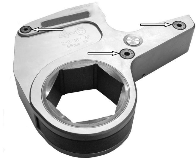
**Figure 6. Three Off Shoulder Screws**
