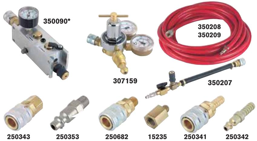
**No. 307159** – Pressure reducing valve. Allows use of bottled gases to operate jacks (works on CGA-580 Nitrogen/Argon/Helium bottles). Contains standard bottle fitting on inlet and 1/4" industrial interchange (female) outlet. Wt., 4 lbs.
