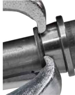
Tapered roller bearing on shaft.
