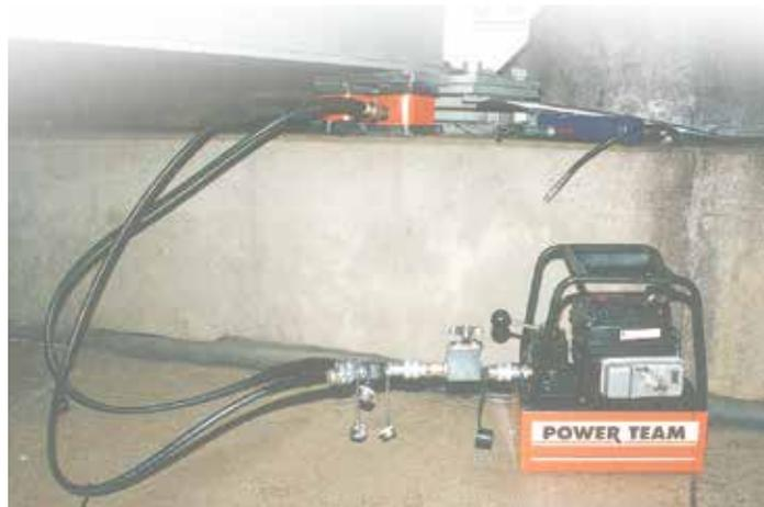
**Gasoline Powered Hydraulic Pumps like this PG303 help provide hydraulic force at remote locations.**
