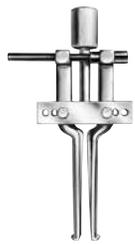
**Internal pulling attachments** have narrow jaws which extend through the center of the part to be pulled. They provide a straight pull and avoid damaging housings. Internal attachments feature adjustable jaws to fit various diameter parts. (page 204)
