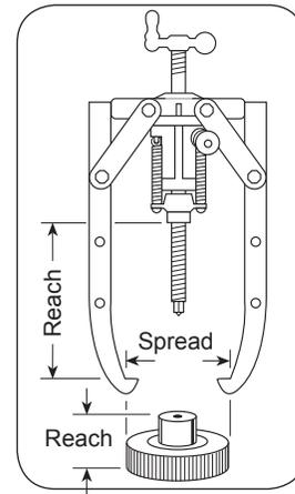
**CAUTION:** Always use a 3-jaw puller where clearance permits in order to provide a more stable setup and a more even pulling force.
