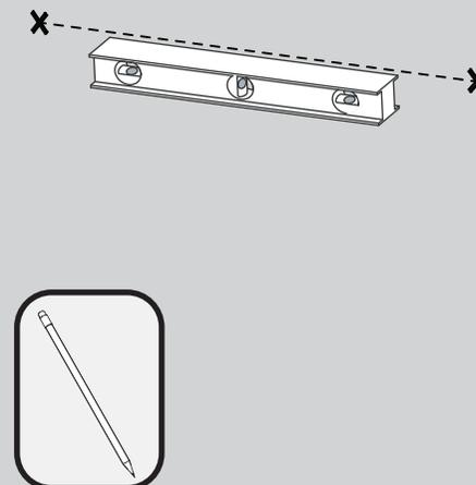
**3** Align Mounting Plate over center point marked in previous step. Mounting Plate should be vertical with Notch in the cylinder (1) pointing to the bottom as shown below. Mark Mounting Screw locations onto the wall surface. Remove items after marking mounting locations.
