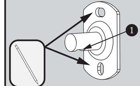
**4** If mounting directly to wood stud, Plastic Anchors are not required. If mounting to tile, acquire proper mounting hardware capable of supporting the accessory in use. If mounting to drywall, drill guide holes at marked locations using a Drill equipped with a  $\text{Ø}3/16"$  bit.
