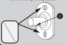
If mounting directly to wood stud, Plastic Anchors are not required. If mounting to tile, acquire proper mounting hardware capable of supporting the accessory in use. If mounting to drywall, drill guide holes at marked locations using a Drill equipped with a Ø 3/16" bit.
