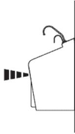
2. As the user enters the beam's effective range, the beam is reflected back into the sensor receiver and activates the solenoid valve. Tempered water flows from the faucet into the sink until the user is no longer detected.
