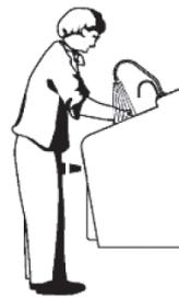
3. When the user moves away from the sensor, light is no longer reflected to the sensor. An electrical signal then deactivates the solenoid valve, stopping the water flow. The circuit then automatically resets and is ready for the next user.
