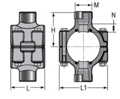
Bolt = 10 Torque FT./LBS. Hole Size = 2-1/4
