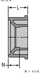
**Type** Flush Bushing **Connection** Spig x Hub
