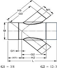
Reducing Type Connection Socket x Socket x Socket
