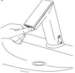
Cover IR clic until LED flashes 4x - hold on until LED flashes 1x to 8x, from minimum to maximum. See diagram below. Release when requested range is reached.
