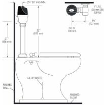
The Model 8116 valve is designed for installations where the water supply is roughed-in 27" (686 mm) above the top of the water closet.
