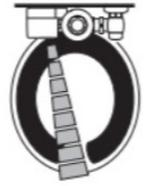
2. As the user enters the beam's effective range, 8" to 54" (203 mm - 1372 mm), the Object Lock Infrared Sensor senses the user.
