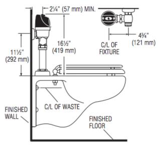
When installing the Optima Plus in a handicap stall: Per the ADA Guidelines (section 604.9.4) it is recommended that the grab bars be split or shifted to the wide side of the stall.
