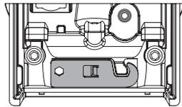
Insert spray removal tool into spray slot by sliding hook end of key between faucet spout and insert. Pull insert out of faucet once hooked.
