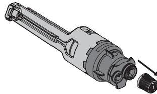
Insert new solenoid caddy at a 45° angle.
