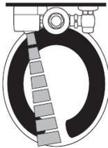
2. As the user enters the beam's effective range, 22" - 42" (559 mm-1067 mm), the object lock infrared sensor senses the user.
