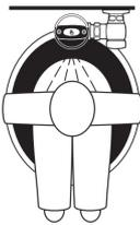
2. As the user enters the beam's effective range (22" to 42") the beam is reflected into the OPTIMA Plus Scanner Window and transformed into a low voltage electrical circuit. Once activated, the Output Circuit continues in a "hold" mode for as long as the user remains within the effective range of the Sensor.
