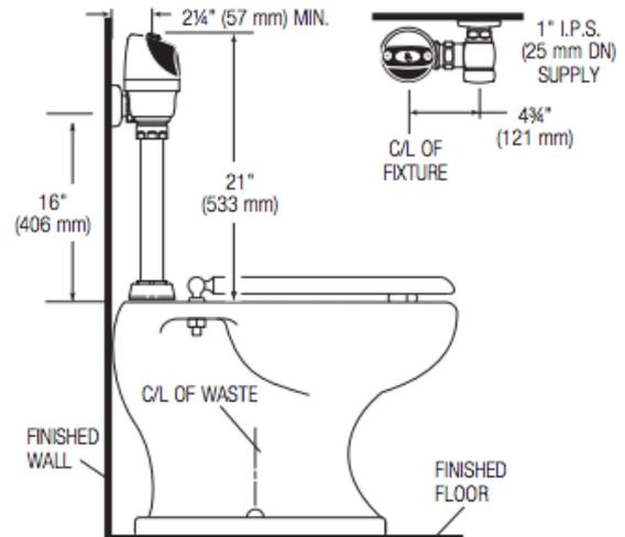
When installing the G2 Optima Plus in a handicap stall: Per the ADA Guidelines (section 604.9.4) it is recommended that the grab bars be split or shifted to the wide side of the stall. If grab bars must be present over the valve, use the Alternate ADA Installation as shown to the right.
