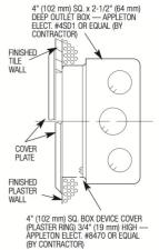
To ensure a perfect rough-in, Sloan recommends the use of the EL-485-A Flushometer Electrical Box Positioning and Support Kit. Specify and order the EL 485-A Kit separately. Consult factory for installation details.
