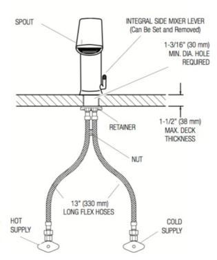
When the BASYS Series faucet is installed on a sink that has three (3) hole punchings, a Base Plate should be used. Base Plates should be specified at time of order.
