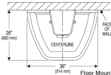
**NOTE:** When both a Rim Height of less than 34" (864 mm) and ADA Compliancy is required, the Low Profile Cabinet must be selected.
