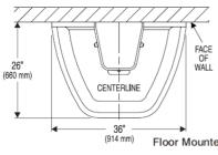
NOTE: When both a Rim Height of less than 34" (864 mm) and ADA Compliancy is required, the Low Profile Cabinet must be selected.
