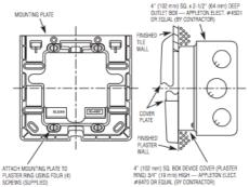
Failure to properly position the electrical boxes to the plumbing rough-in will result in improper installation and impair product performance. All tradesmen (plumbers, electricians, tile setters, etc.) involved with the installation of this product must coordinate their work to assure proper product installation. Installation Template furnished with Flushometer.
