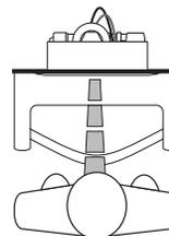
3. When the user steps away from the OPTIMA Sensor, the loss of reflected light initiates an electrical "one-time" signal that energizes the Solenoid Operator, and activates the Flushometer to flush the fixture. This occurs on the water closet approximately three (3) seconds after indication. This delay is built into the Sensor to help prevent false flushing due to movement by the user. The circuit for both water closets and urinals then automatically resets and is ready for the next user.
