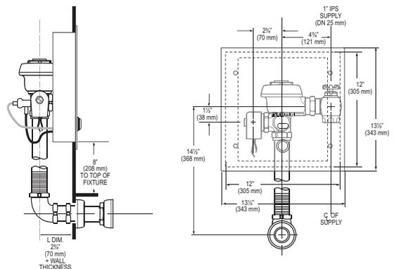
‡ POSITION OF SENSOR BOX CAN BE RAISED OR LOWERED 1" (25 mm) IF IN CONFLICT WITH HANDICAP GRAB BARS.
