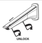
Place new crown on faucet by sliding onto spout and tightening hex screw on underside of spout.
