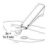
Cover IR clic until LED flashes RED 4 times - hold IR clic on until LED flashes 1 time to 8 times from minimum to maximum range. See diagram below. Release when requested range is reached.
