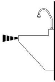
2. As the user enters the beam's effective range, the beam is reflected back into the sensor receiver and activates the solenoid valve. Tempered water flows from the faucet into the sink until the user is no longer detected.
