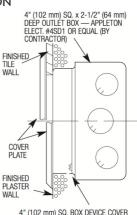
4" (102 mm) SQ. BOX DEVICE COVER (PLASTER RING) 3/4" (19 mm) HIGH – APPLETON ELECT. #8470 OR EQUAL (BY CONTRACTOR)
